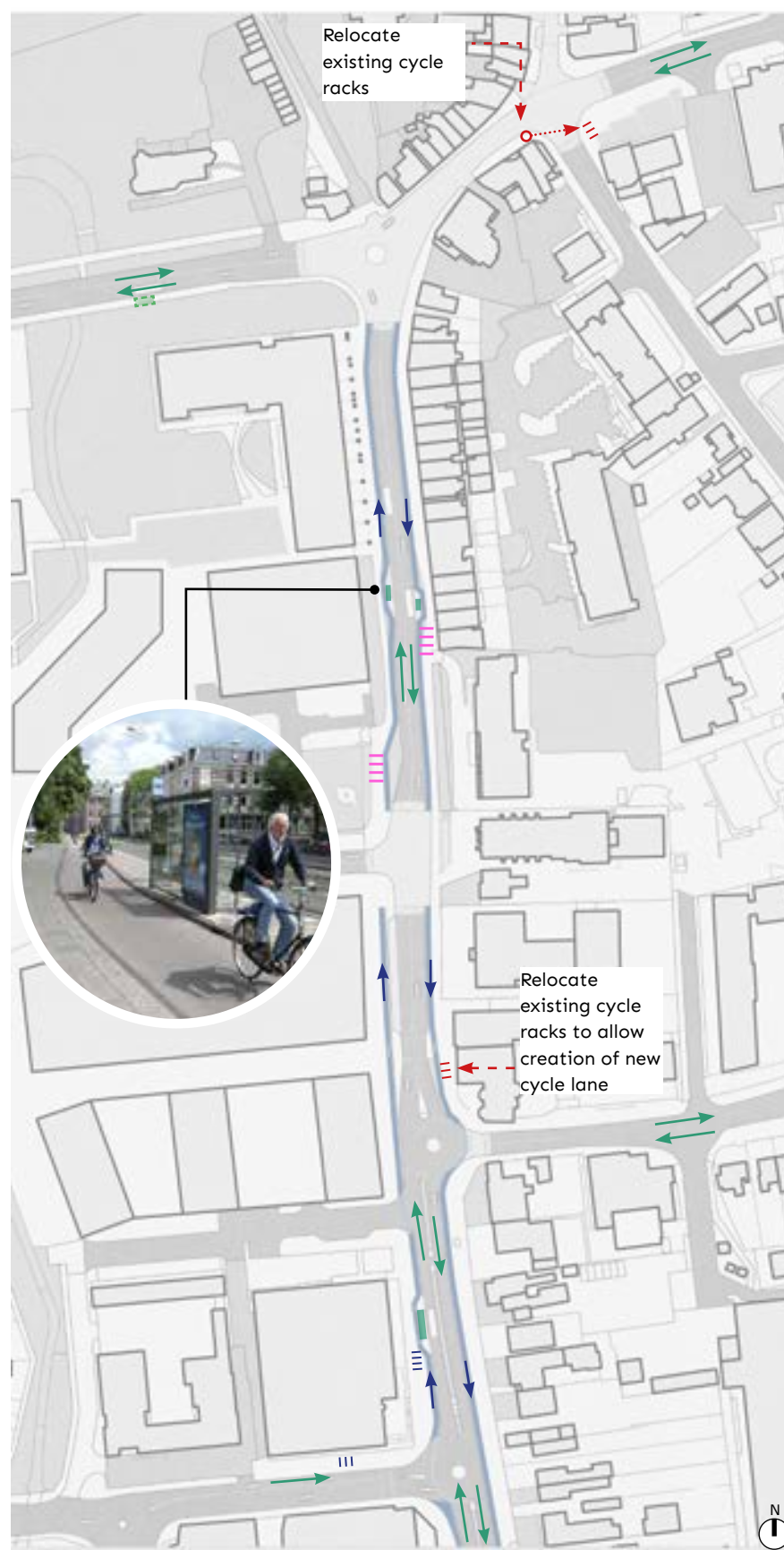
Upper Marlowes map - existing bus and cycle routes New cycle lanes Existing bus routes retained bus stop to be relocated existing bus to be maintained new cycle lane (MAT 05) existing cycle racks to be maintained existing cycle racks to be relocated new cycle racks
