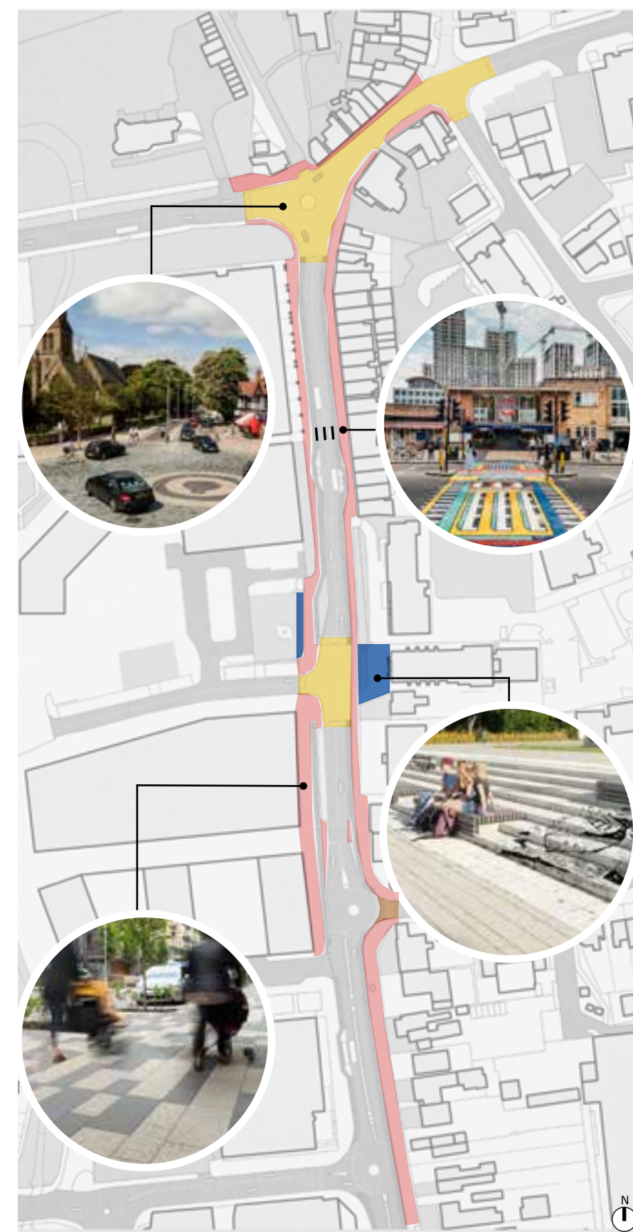
Upper Marlowes map - road and pavement surface new shared surface area existing finish of pavement (asphalt or slabs) to be replaced with new paving slabs level street crossing removal of existing retaining wall and adjustment of ground levels. Creation of new steps, seating areas and new paving
