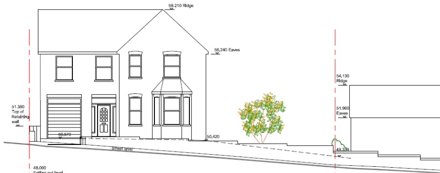
Front Elevation as existing (Street View) Scale - 1:100
