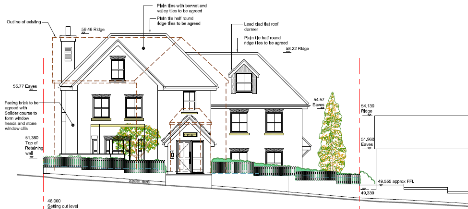
Front Elevation as proposed (Street View) Scale - 1:100
