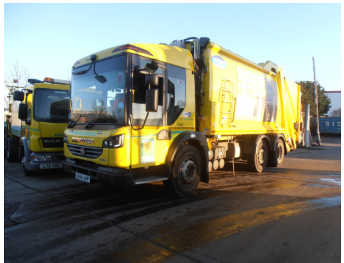
Figure 4.1.2 Image of lorry used by Dacorum Council to collect waste. This measures approximately 10m x 3m. All residential layouts must consider size and manoeuvrability of this vehicle.
