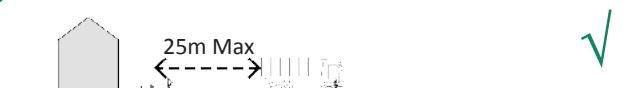
Figure 4.1.5 Operatives must walk no further than 25m from the truck to the collection point.
