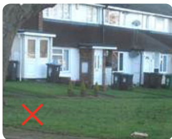
The above example in Hemel Hempstead shows the unsightly views created by inadequate rubbish store provision.
